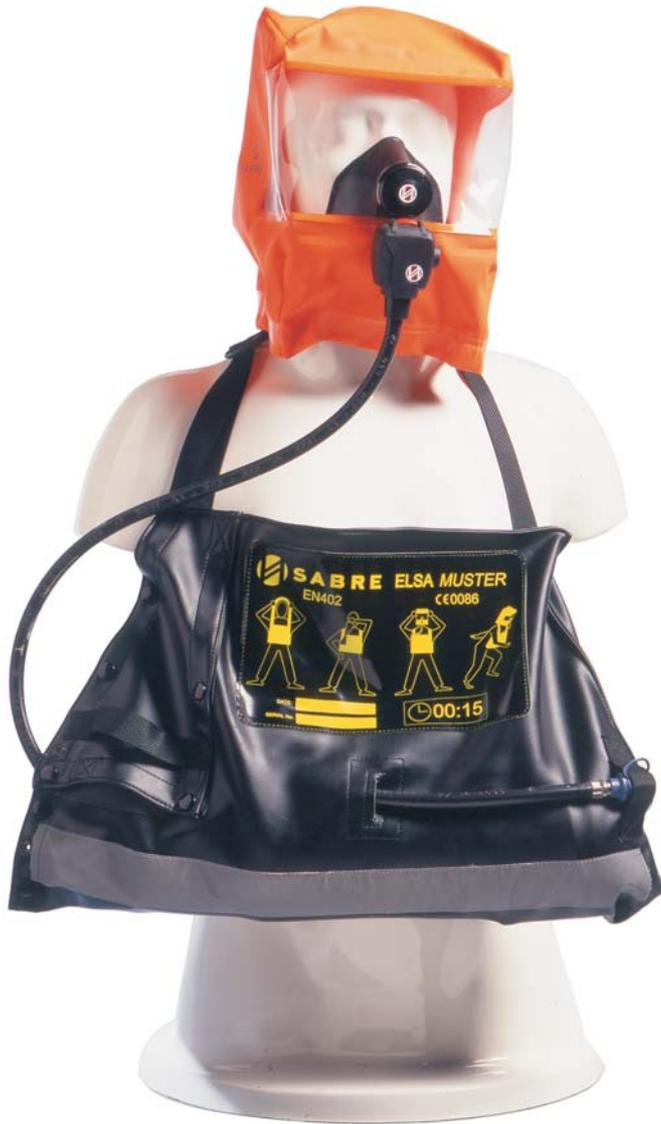
*The Sabre ELSA Muster is an open circuit, positive pressure airline breathing apparatus generally comprising; Anti-static bag, high pressure reducing valve, automatic positive pressure demand valve and coupling for airline supply hose.*
